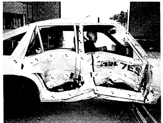
Figure 4. Penetration of stiff longitudinals from weak car with poor frontal interconnections.
