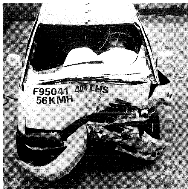
Figure 5. Deformed car after an offset frontal crash test with bottoming-out of the deformable obstacle.
