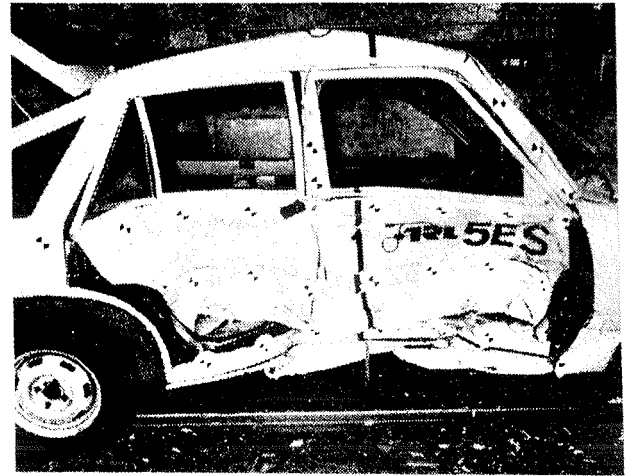
Figure 3. Quite good load spreading from stiff car with well interconnected front structure.
